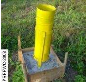
Manual rain gages (top) are a lot cheaper than digital ones but are not appropriate for real-time observations.
