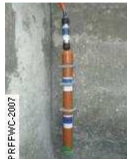
An SMS-enabled, pressure-type river gage, such as the one shown on the left, have been installed in the Binahaan River local flood warning system in Leyte, Philippines.
