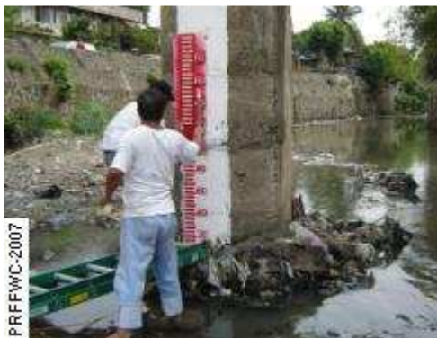
Manually read staff gages (top) are relatively cheaper but requires continuous monitoring during inclement weather condition.
